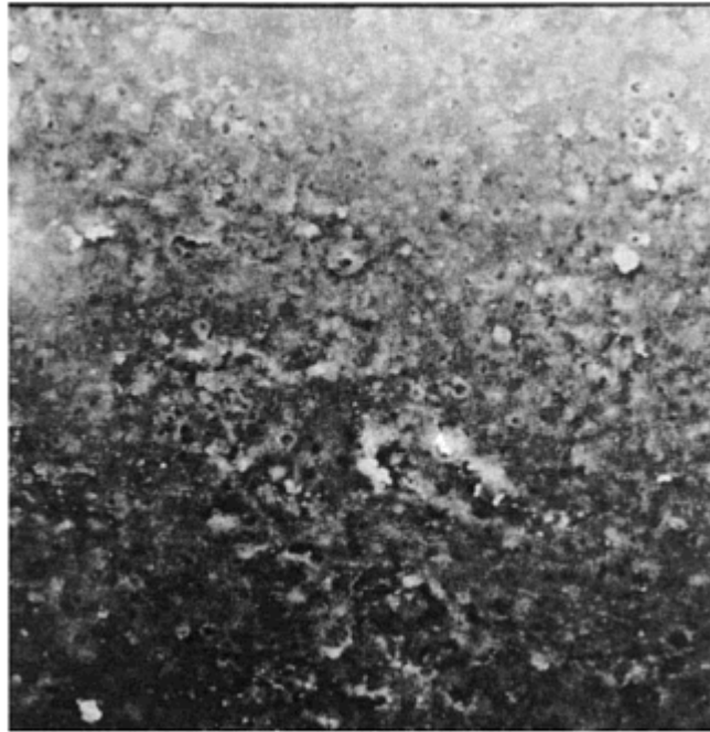
Fig. 13.14 Scanning electron micrograph of an HPMC film produced with a 10° solid cone spray (original= \times 100 ). R_a=1.44\mu\text{m} .
